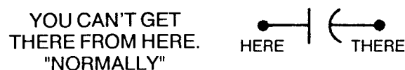
FIGURE 17-25. The Capacitor Symbol Does Not Show A Completed Circuit Between the Terminals.
